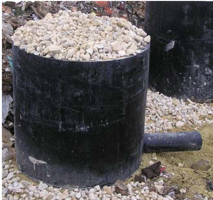
Figure 3 : Lysimeters set up in the landfill cell
