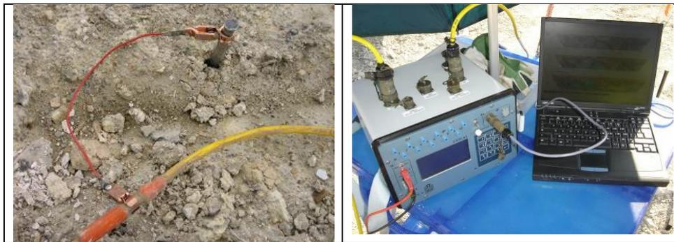
Picture 1 : Experimental set-up of the ERT measurement
