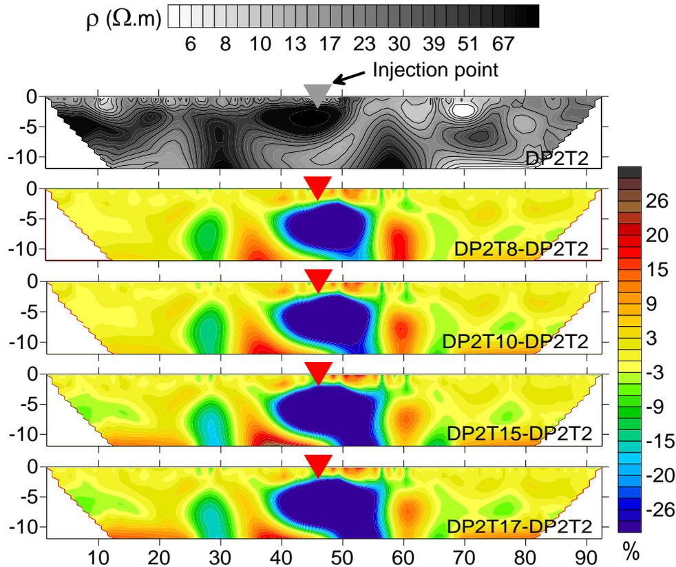
Graph 1 : Preliminary ERT study of the plume of the recirculation system: Interpreted resistivity variations compared with an electrical imaging before the beginning of injection
