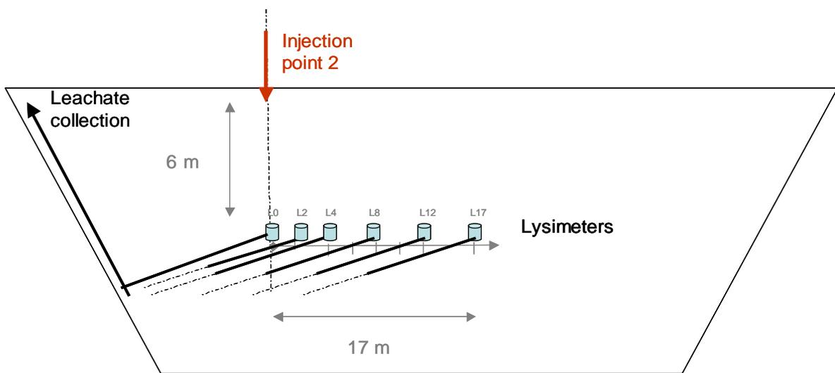
Graph 2 : Plot of the lysimeter set-up (cluster B)
